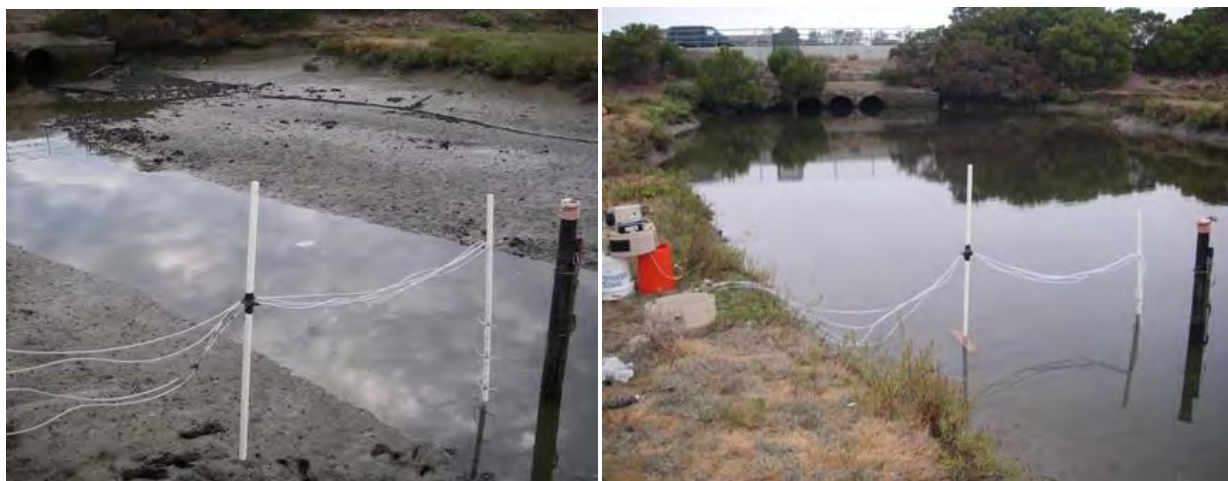
Figure 1.6. Stratification sampling set-up (photos: SMBRC 2010).
