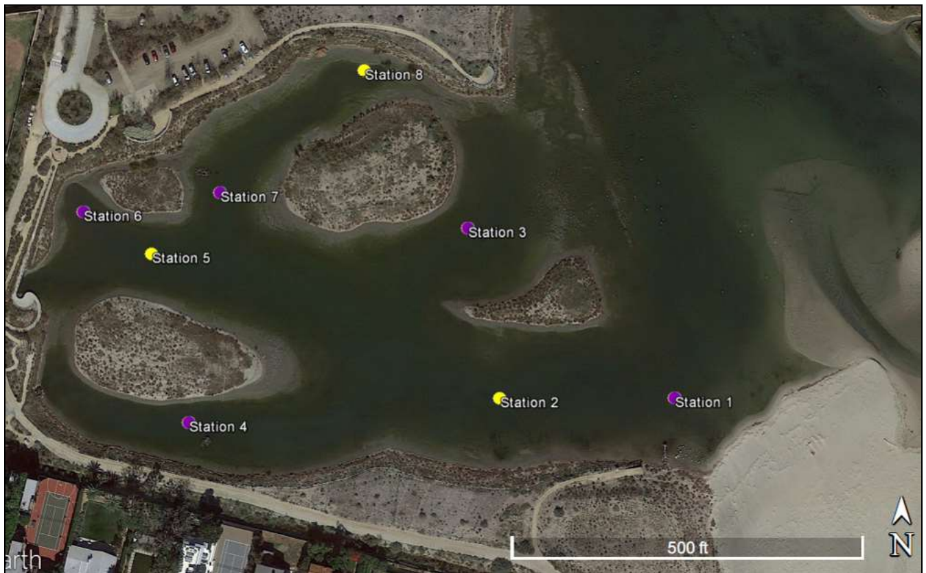
Figure 15. Map of post-restoration vertical profile, SAV/algae, surface and bottom water nutrient, and sediment survey stations. Stations 2, 5, and 8 are the locations of the three permanently-deployed YSI data sondes (in yellow).
