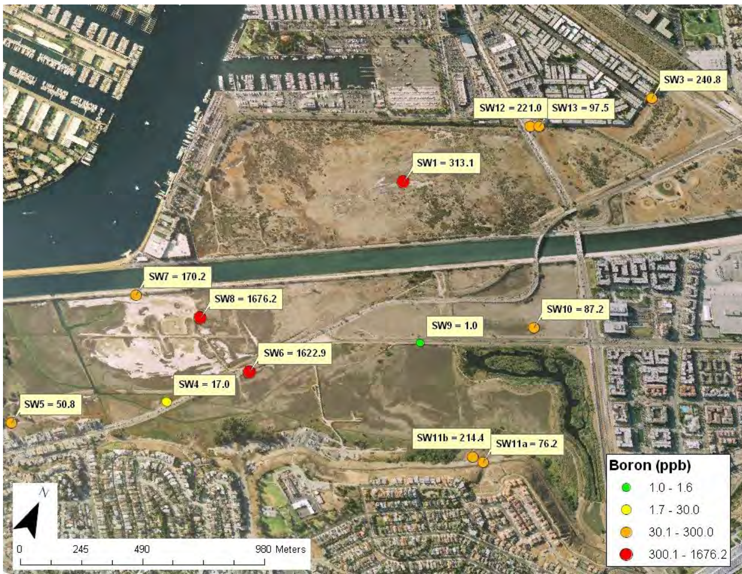
Figure 1.33. Dissolved boron in stormwater samples at all stations. The green dots indicate values below the chronic toxicity value for boron, and the orange and red dots are above the acute maximum toxicity levels (USEPA 2009).
