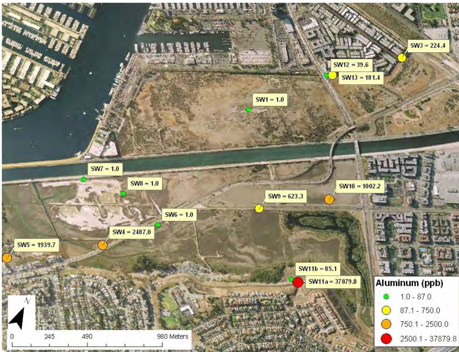
Figure 1.32. Dissolved aluminum in stormwater samples at all stations. The green dots indicate values below the chronic toxicity value for aluminum, and the orange and red dots are above the acute maximum toxicity levels (USEPA 2009).
