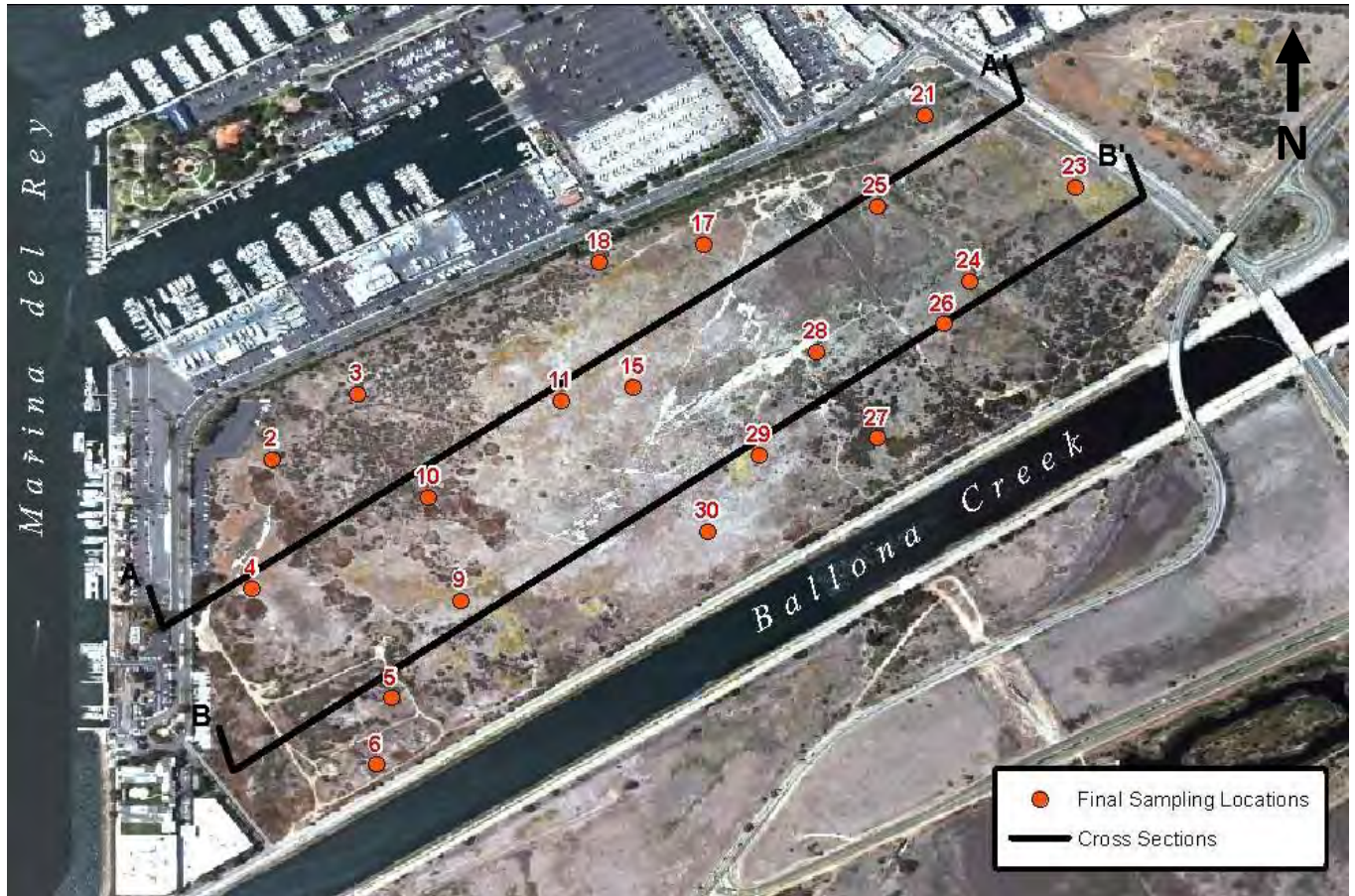
Figure 3.1. Deep borehole core sampling locations in Area A (reproduced from Weston Solutions 2009).
