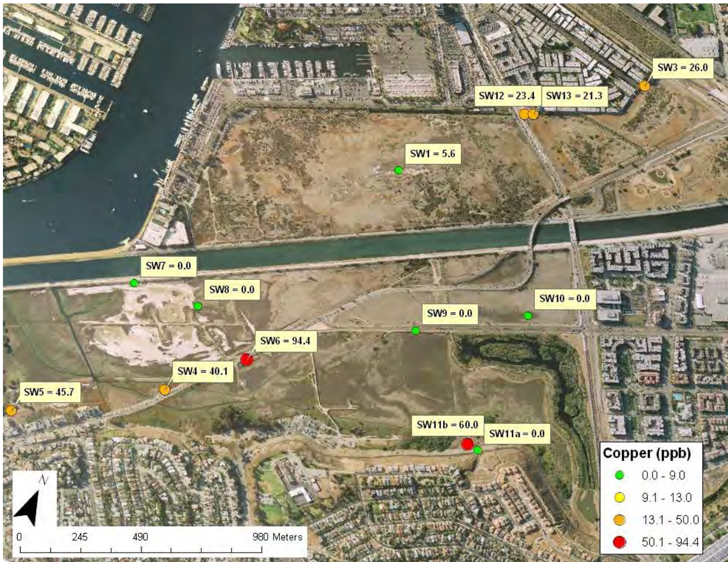
Figure 1.31. Dissolved copper in stormwater samples at all stations. The green dots indicate values below the chronic toxicity value for copper, and the orange and red dots are above the acute maximum toxicity levels (USEPA 2009).
