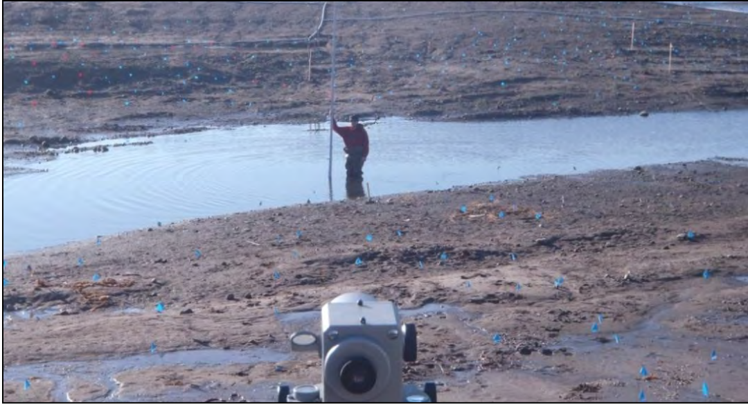
Figure 10. Surveying in the thalweg for the location of a YSI sonde station, post-restoration, February 2013.
