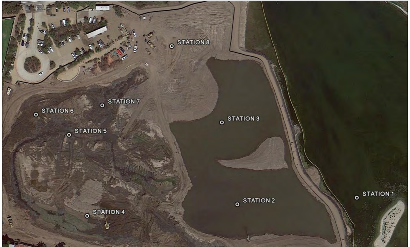
Figure 12. Map of water quality vertical profile and SAV/algae survey stations. Water quality stations 2, 5, and 8 are also the locations of the three permanently-deployed YSI data sondes. Note that each SAV/algae station is comprised of three cross-channel transects approximately 10 meters apart (individual transects not identified on map).
