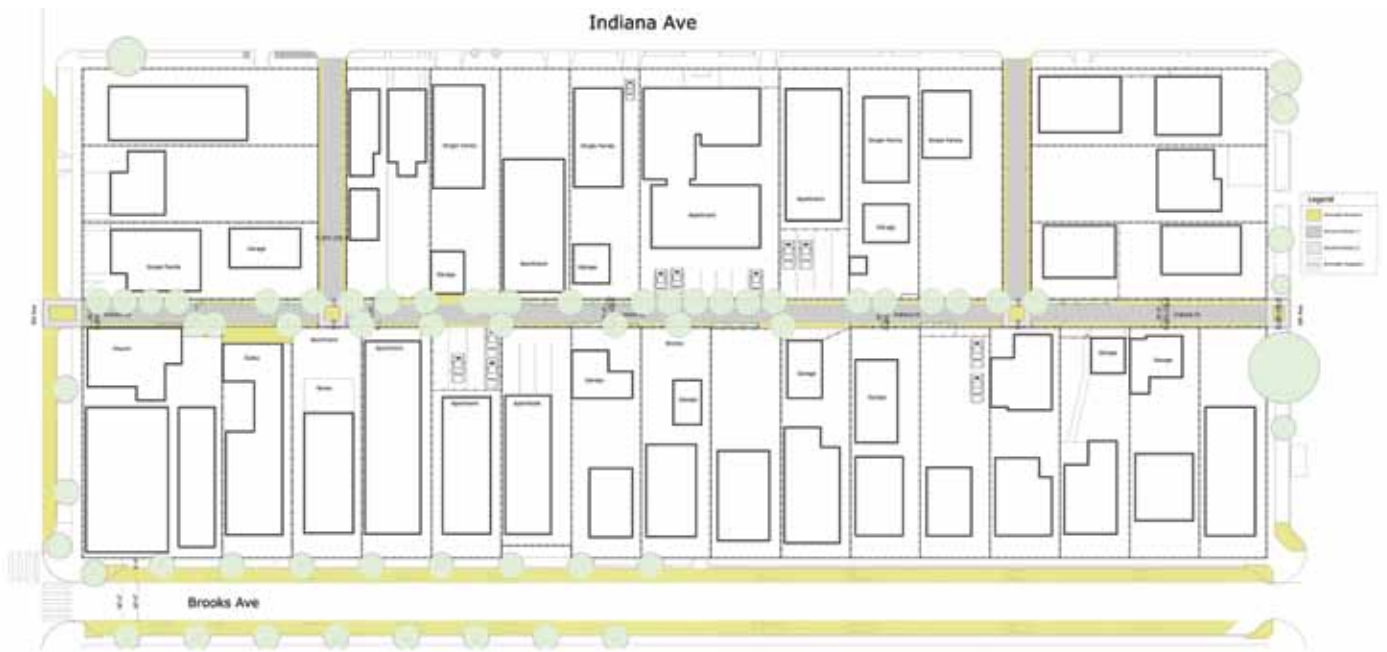
FIG. 21. The plan calls for creating a street tree network to absorb air pollutants and provide shade; paving changes to increase permeability and slow traffic; and widening sidewalks to accommodate pedestrian-oriented activities.
