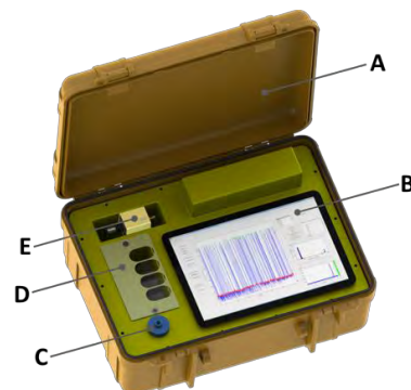
Figure 4.3-3. Conceptual rendering of a ddPCR device. A) Portable brief-case format digital PCR device with external power outlet; B) The tablet PC with control and data analysis; C) The sample injection port; D) The rapid-replace consumable reagent bay; and E) The target primer library. Photo Credit: Cody Youngbull, Arizona State University.
