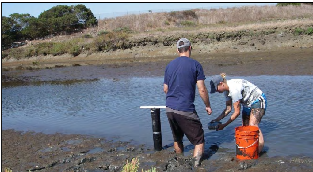
Figure 84. Photograph of benthic invertebrate core sampling in the Area B tide channels.
