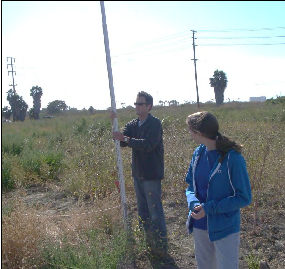
Figure 96. Photograph of engineering students doing an elevation survey in upland habitat types.
