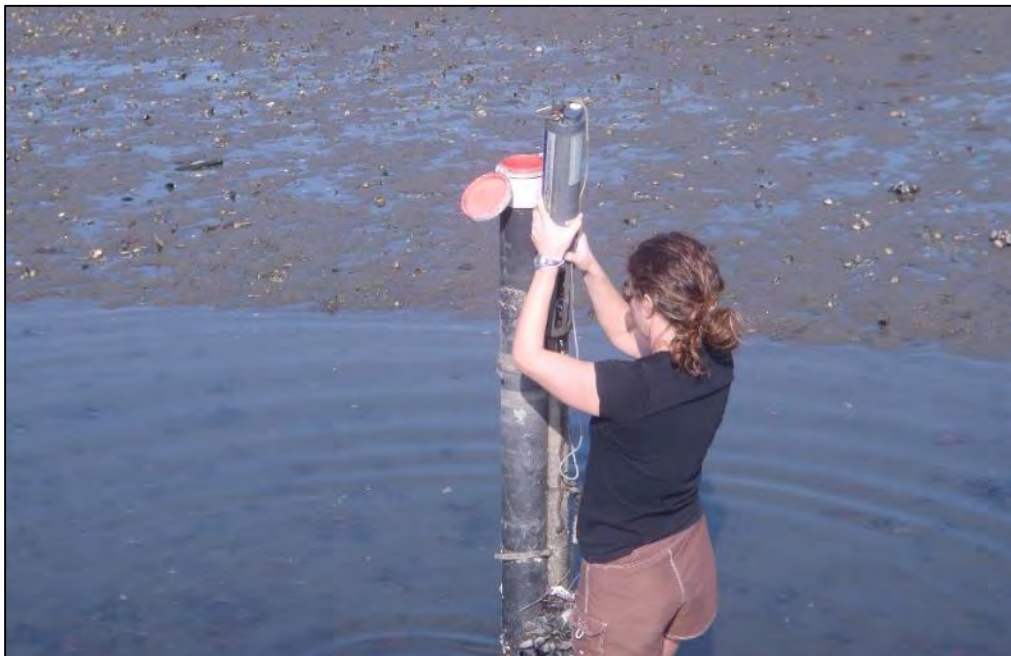
Figure 23. Photograph of data sonde deployment in the main muted tidal channel at Ballona B-W.
