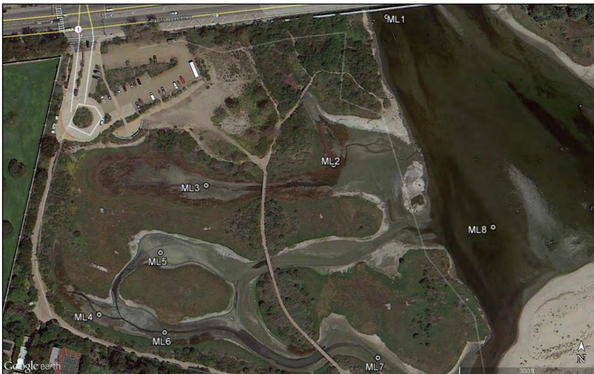
Figure 12. Map of pre-restoration water quality monitoring stations. ML2 and ML6 are the locations of the pre-restoration permanently-deployed YSI data sondes.
