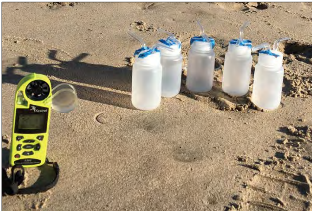
Figure 42. MWAC samplers deployed at restoration site.
