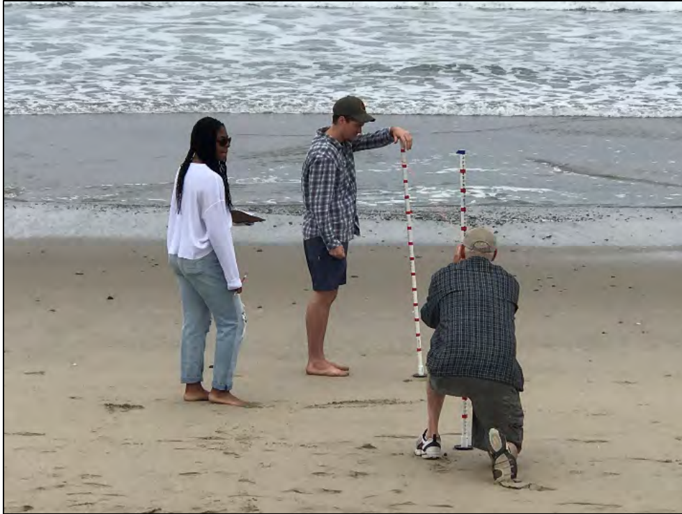
Figure 29. TBF staff and affiliates from LMU's Coastal Research Institute conduct an elevation profile survey (24 May 2018).
