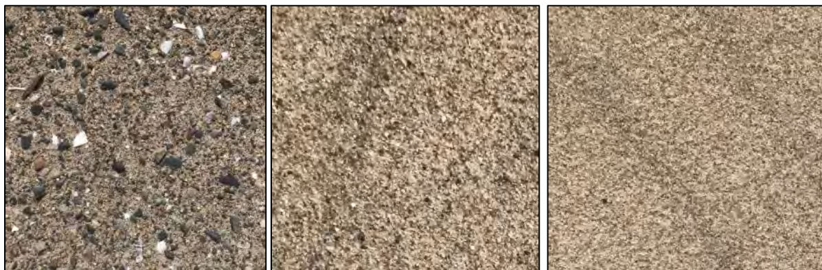
Figure 41. Sand grain examples in restoration site [left: pebbles (very fine); middle: course sand; right: fine to very fine sand].
