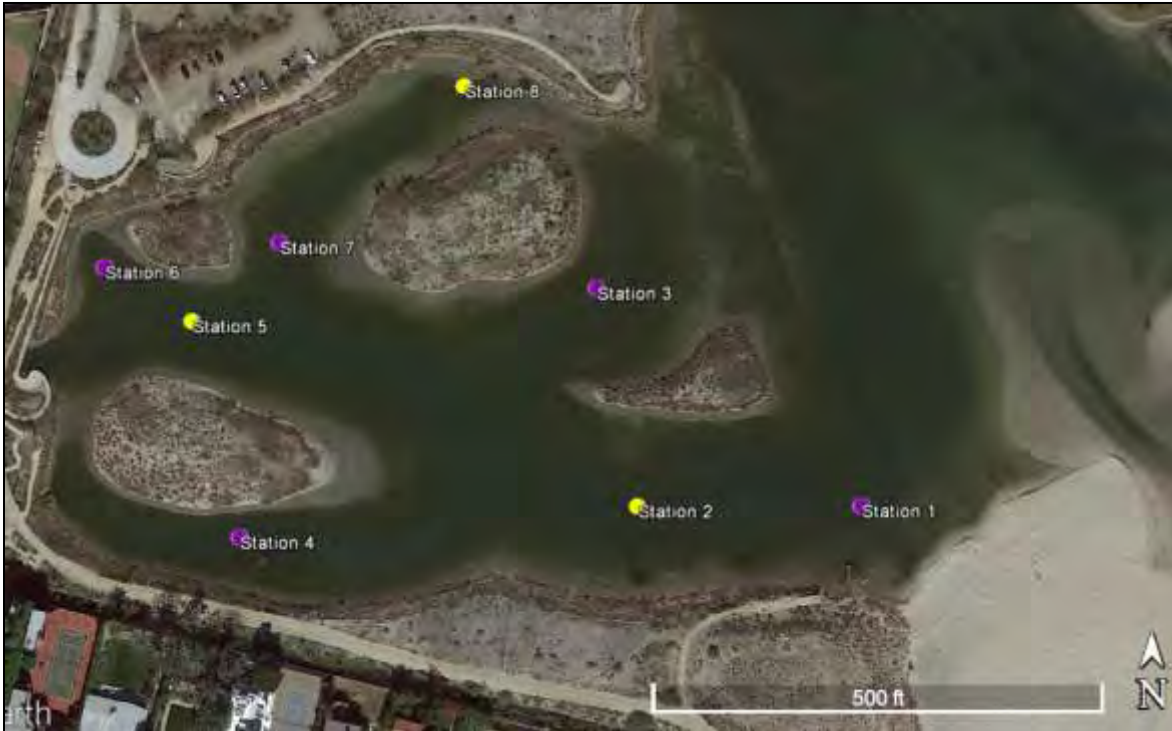
Figure 29. Map of post-restoration vertical profile, SAV/algae, surface and bottom water nutrient, and sediment survey stations. Stations 2, 5, and 8 are the locations of the three permanently-deployed Hydrolab data sondes (in yellow).
