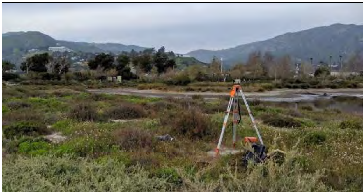
Figure 20. Cross-channel elevation survey at Malibu Lagoon on 22 February 2019.
