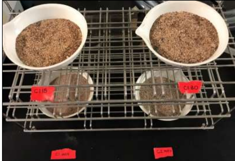
Figure 43. Organics (loss on ignition) analysis on sand samples (18 July 2018).
