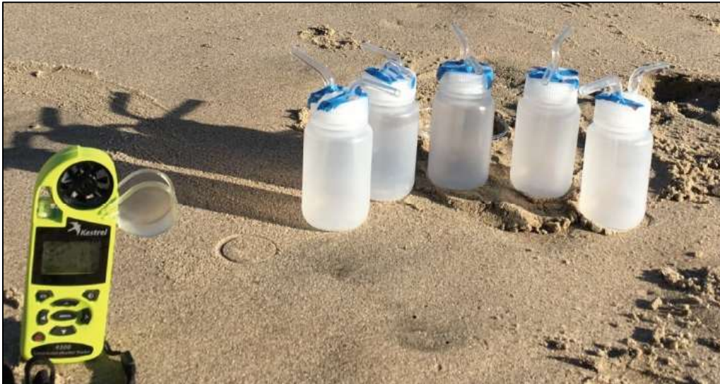
Figure 42. MWAC samplers deployed at restoration site.
