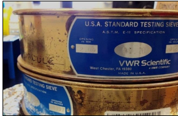
Figure 4. Stacked sieves of decreasing screen size.
