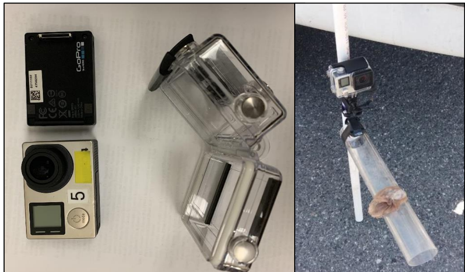
Figure 1. Go Pro camera (bottom left) with the battery extender (top left) and the waterproof case that attached to the PVC apparatus (middle); baited camera PVC T-frame setup (right).
