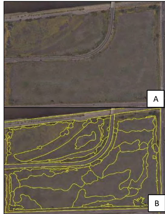
Figure 5. Example of vegetation stands with indistinct or difficult aerial signatures (A) and the delineation resulting from walking transition boundaries (B).
