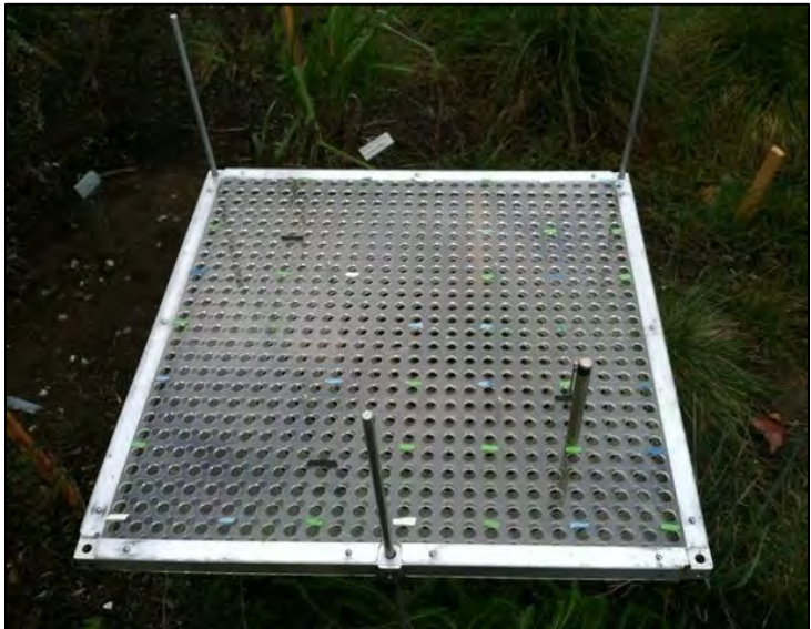
Figure 2. Laser quadrat (0.5m x 0.5m) and laser pen with taped holes for increased accuracy.
