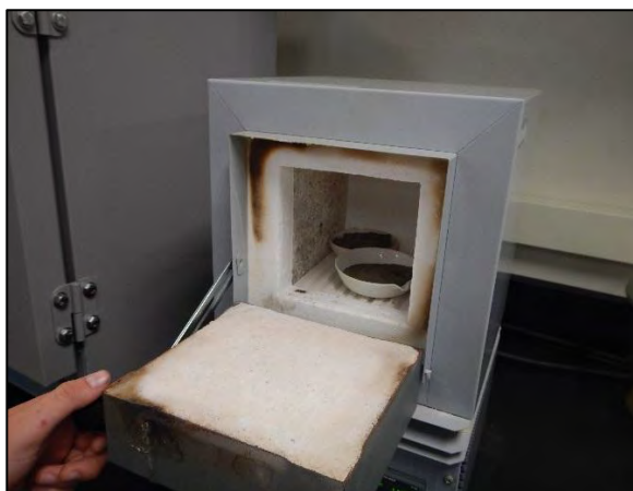
Figure 5. Place crucible carefully in furnace.
