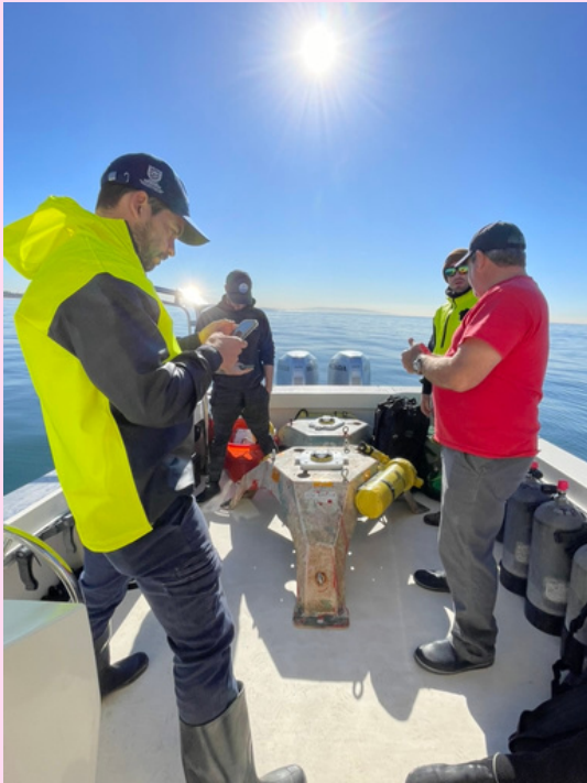
2024: UCLA's Coastal Flood Lab and The Bay Foundation placing a temporary current sensor by the breakwater. Source: UCLA's Coastal Flood Lab
