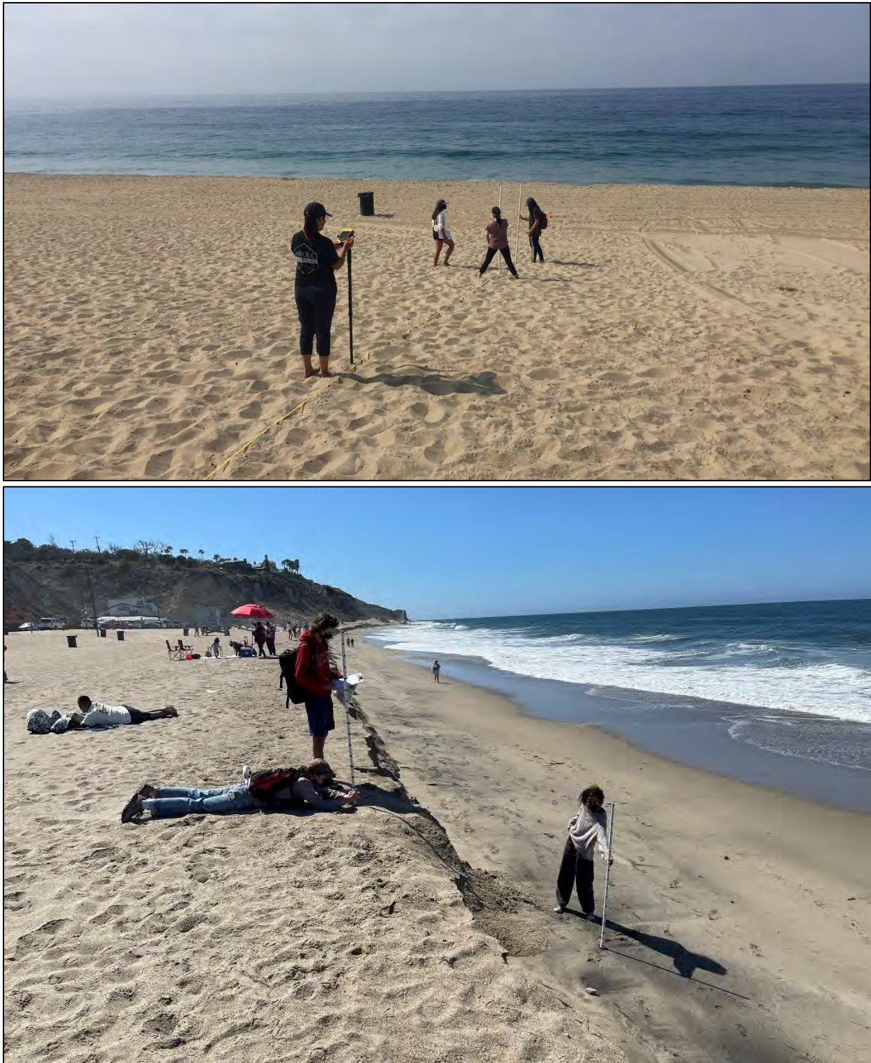
Figure 42. Photos of TBF staff and interns performing elevation surveys using a GPS Trimble and elevation poles.
