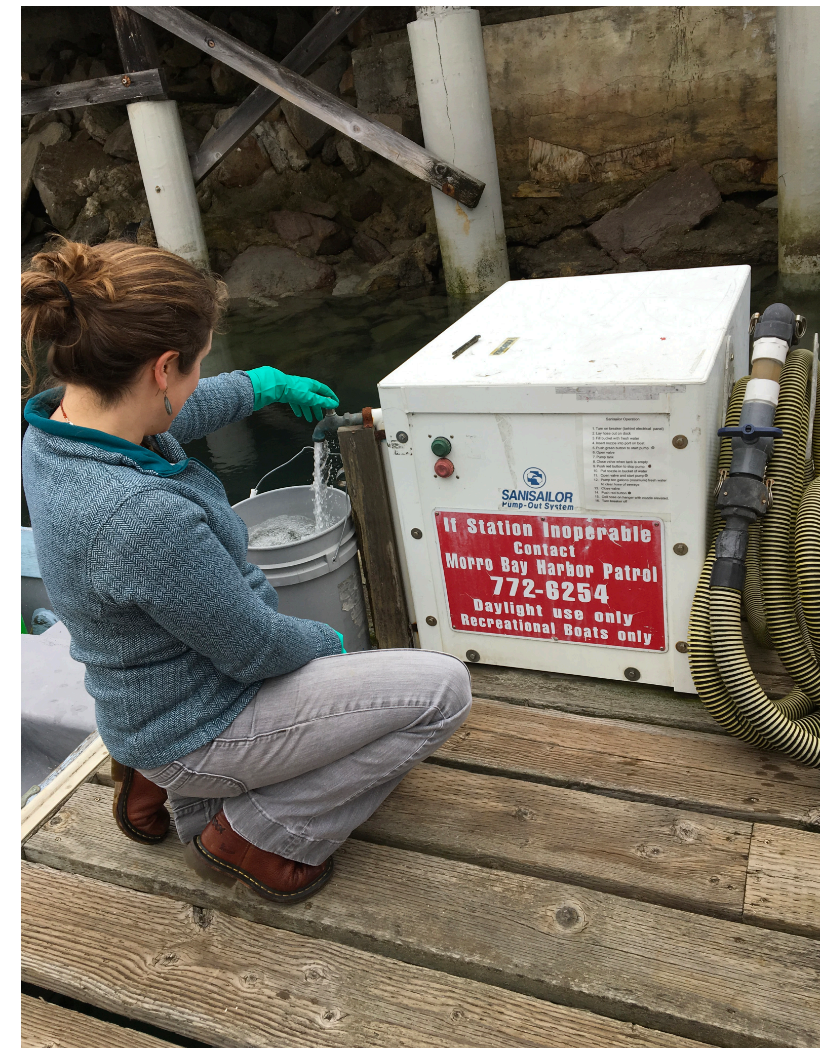
MBNEP staff filling 5-gallon bucket in order to test vacuum time Photo by MBNEP
